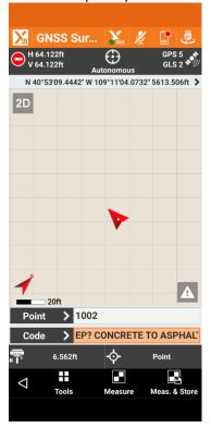
The "?" delimits the Code and Description resulting in a stored measurement and point with a Code property of 'EP' and a Description property of 'CONCRETE TO ASPHALT':
